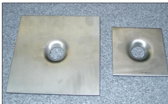
*FIGURA 14- ANGOLI D'ANGOLO E PLASTRE IMBUTITE*
